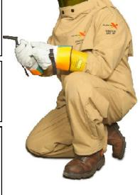
Oberon's ARC65 suit is designed to provide protection from arc flash heat exposures. The suit exceeds the requirements of NFPA 70E Hazard Risk Category 4 (HRC4), up to 70 cal/cm². Oberon's ARC65 suit is manufactured with 80% inherently FR aramid, and 20% melamine. These high technology lightweight (up to 50% lighter than FRT fabrics) and proprietary fabrics can reduce heat stress. All materials used in the construction of these garments are inherently flame resistant, including the thread.
